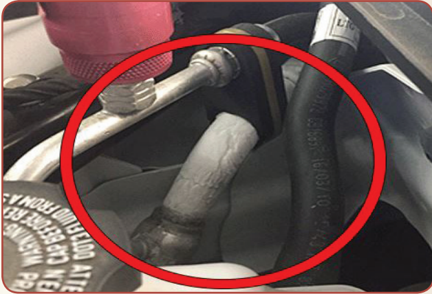
Ice on evaporator core tube
