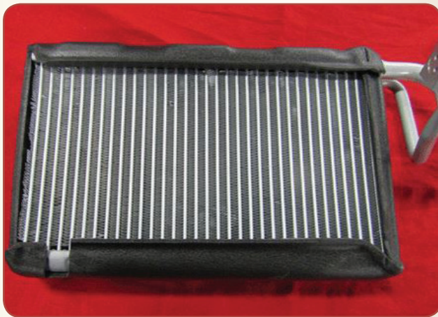
Evaporator core seal around the evaporator core
