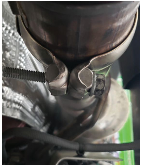
Replace the clamp if bottomed out.
