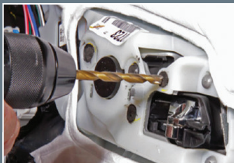
Drill out the four heat stakes to release the handle assembly.
