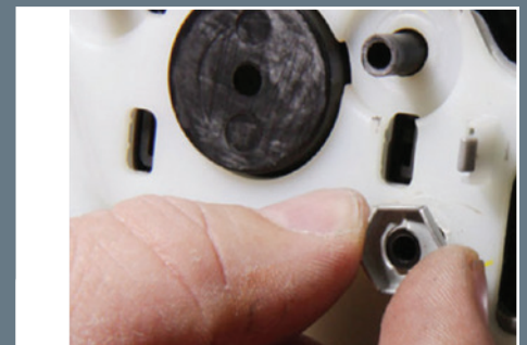
The new door handle is secured with stamp nuts.
