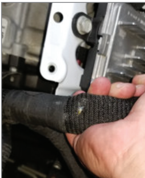
Wiring harness damage from rubbing on the battery tray support bracket for the TCM.
