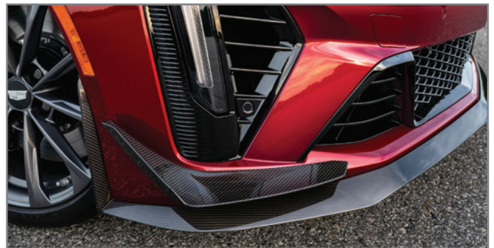
Available carbon fiber packages further reduce lift.
