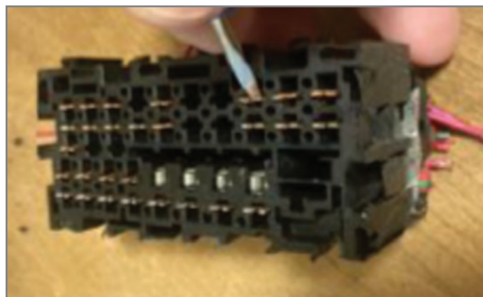
Remove the terminal from the damaged cavity.
