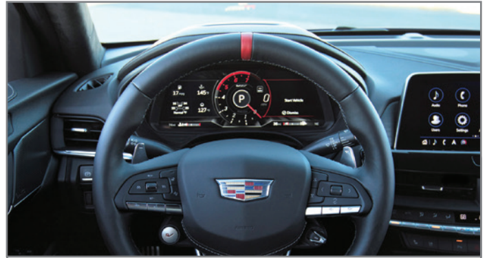
Tap Shift/Manual Mode is activated using the integrated magnesium paddle shifters.
