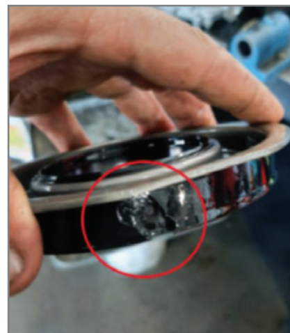
Damage along the side of the forward clutch piston
