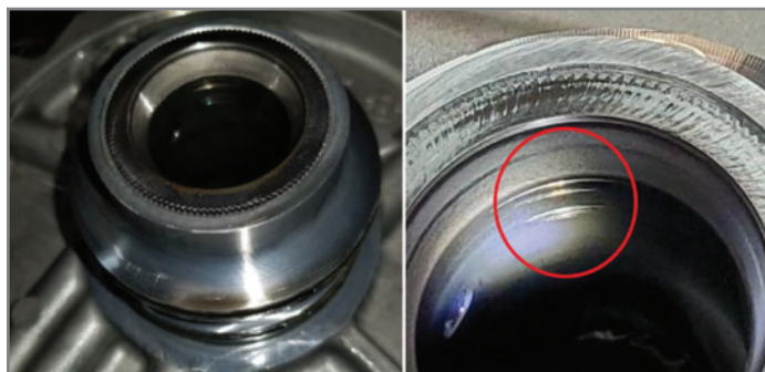
Inspect the pump for signs of internal wear.
