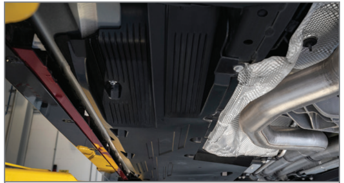
Aerodynamic elements, such as mid-body panels, direct airflow around the vehicle.
