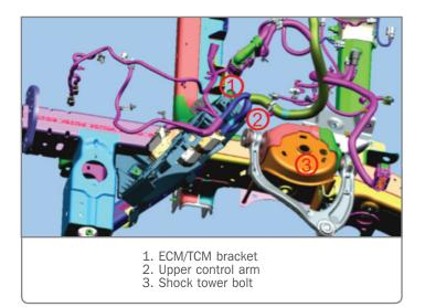
For upper control arm contact, wrap the wiring harness in the harness sleeve and anti-abrasion tape. Secure the harness to the harness clip above the ECM/TCM bracket.
