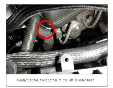
Repair any damaged wiring found by following the wiring repair procedures in the appropriate Service Information. Once repairs are completed, protect and reposition the engine wiring harness to prevent future damage.
