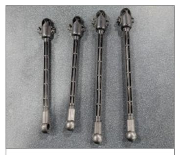
The factory suspension height sensor links are not adjustable.
