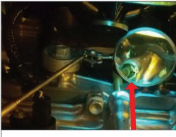
Check for an oil leak from the dipstick tube O-ring.
