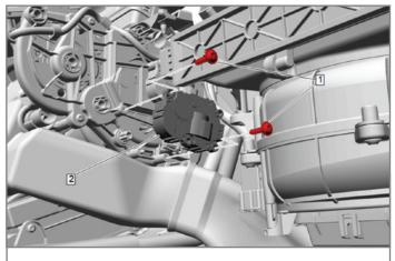
Programmable temperature valve actuator – right side on the 3.0L engine
