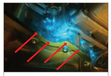
Black light and tracer dye identify an oil leak from the composite oil pan sealing surface.
