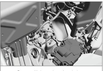
Programmable temperature valve actuator – left side on the 3.0L engine
