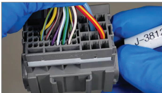
Check for any loose terminals in the X270 harness.
