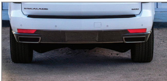
Reverse Automatic Braking uses one or two Short Range Radar Sensors and the ultrasonic Parking Assist Sensors to identify objects behind the vehicle.
