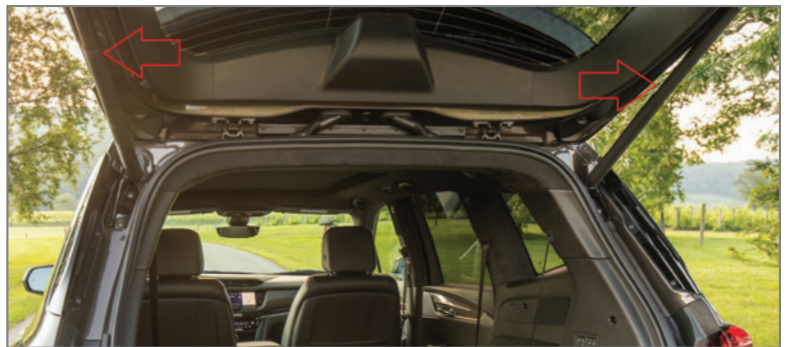
Any residue on the struts is not a fluid leak.
