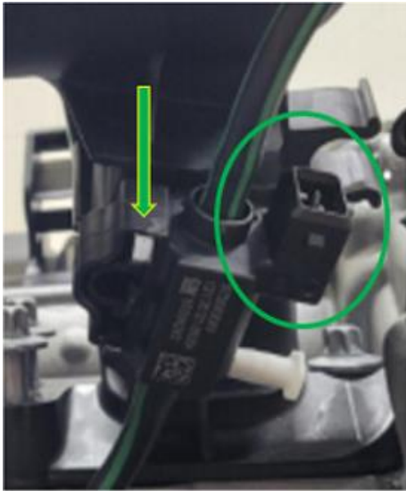
Solenoid connector correct installation retainers latched Keyed section of intake almost even with solenoid
