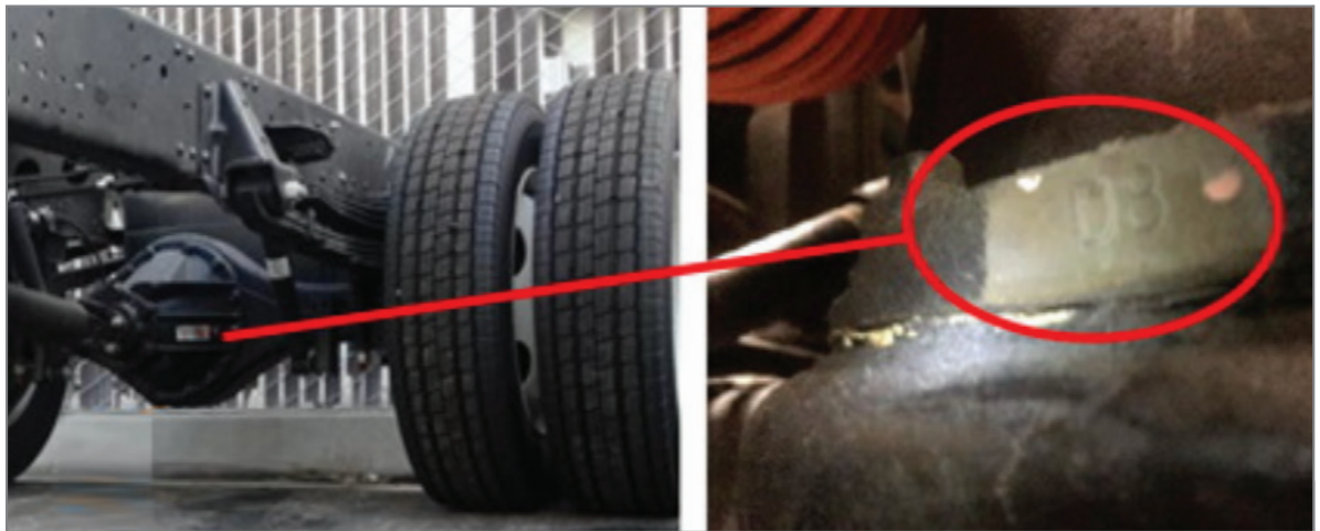
Verify the vehicle is equipped with a limited-slip rear axle by checking the LSD stamp code on the axle.
