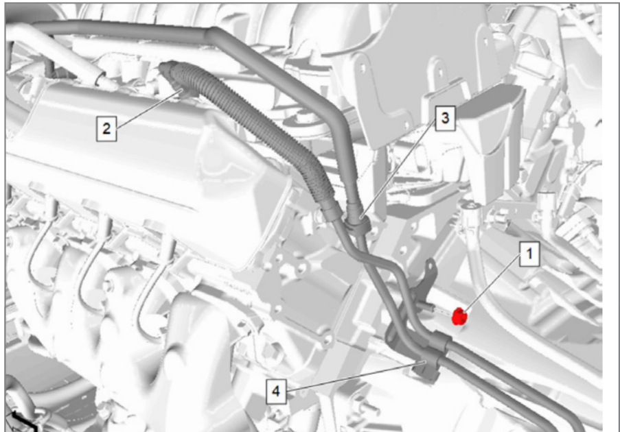
Debris may be causing a restriction in the fuel feed pipe.
