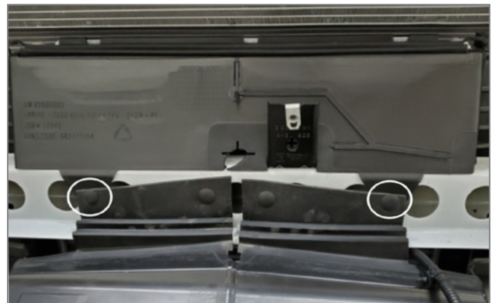
Install the new radiator air front lower baffle behind the outermost tabs of the front bumper lower air baffle.
