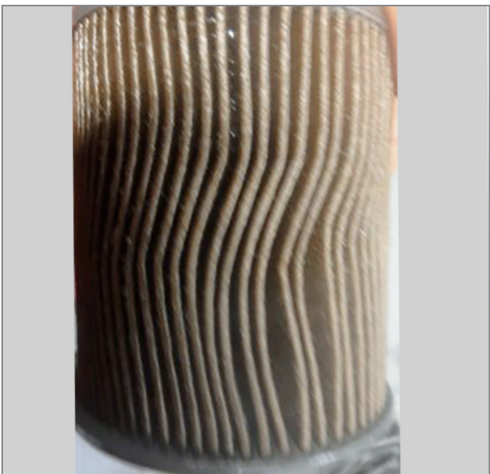
Look for visible metal particles in the oil filter pleats.
