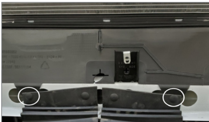
Install a lower air baffle to help reduce CAC icing.
