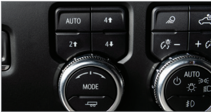
Transfer case controls
