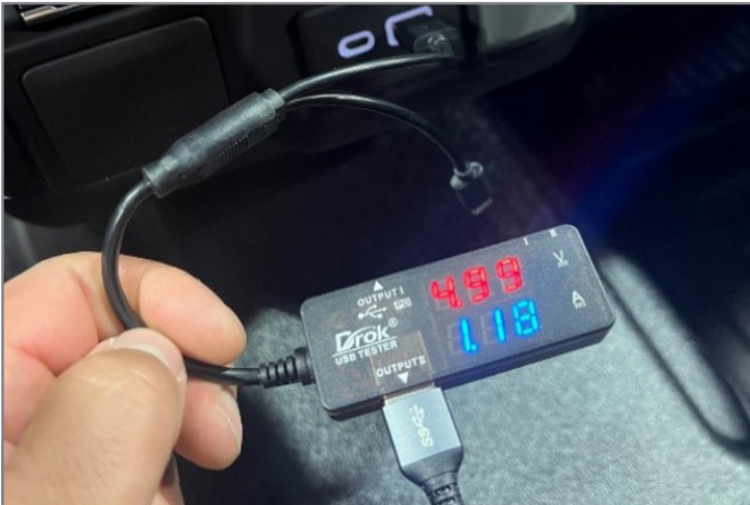
Check for proper voltage using a USB meter.
