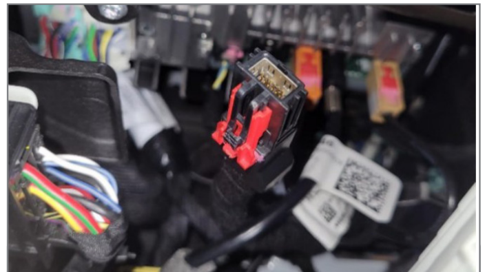
Mini-B USB or 6-pin power connector from the back of the radio
