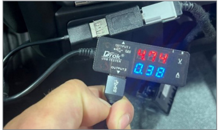
With a USB-A female to mini-B female adapter connected to the mini-B connector, verify if music can be played.
