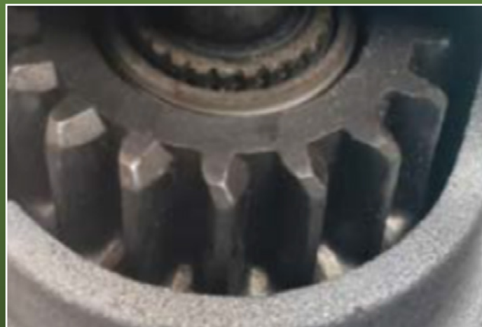
Starter pinion teeth without damage
