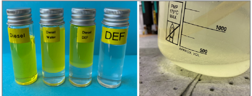
A fuel sample will show a separation of DEF and water from diesel fuel.
