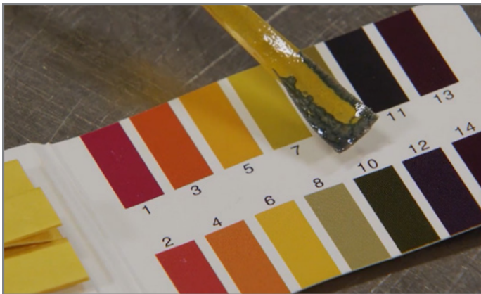
Diesel fuel mixed with DEF
