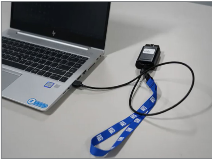
The SAVI dongle can be connected to a PC using the provided USB cable.
