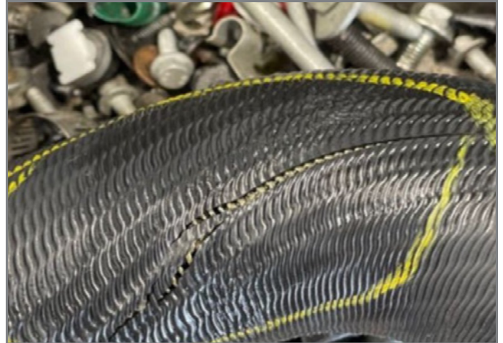
Area shows damage to the inner hose beneath the anti-abrasion sleeve.
