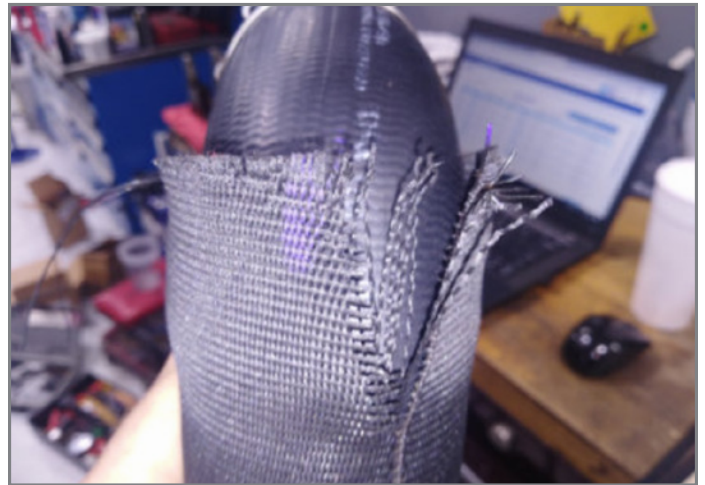
Check for any splitting or damage to the anti-abrasion sleeve.
