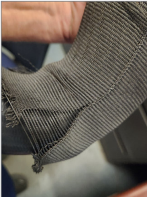
Anti-abrasion sleeve on the charge air inlet pipe
