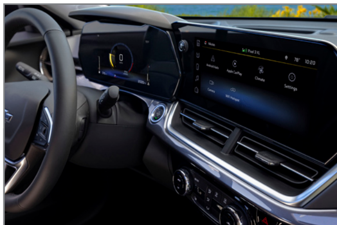
The new design features only one module for the instrument cluster and radio.
