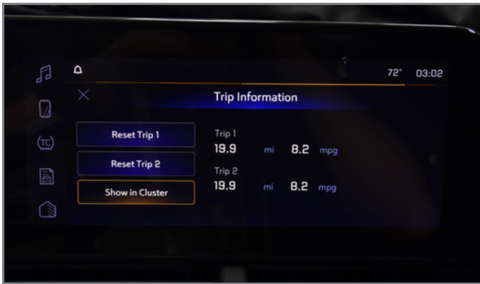
Select Show in Cluster to view information on the instrument cluster display.
