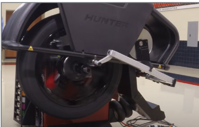
Road Force measurements are used to determine proper alignment of the tire to the wheel.
