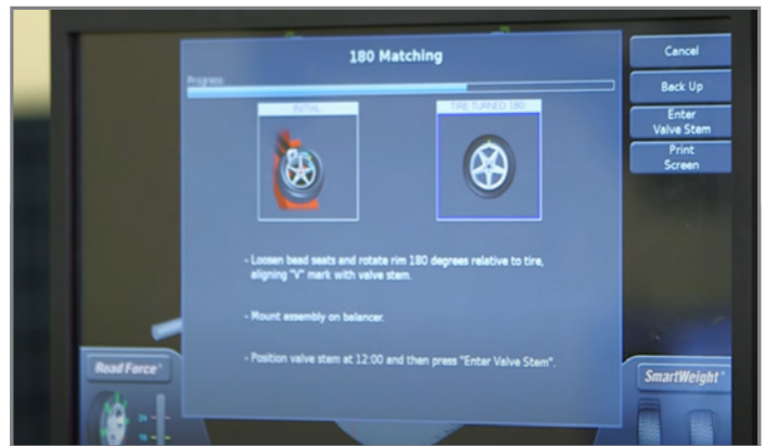
Force Matching can cancel radial force vibration
