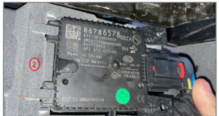
Correctly installed Side Object Detection Module
