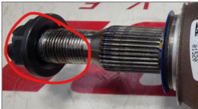
Damage to the wheel drive shaft threads
