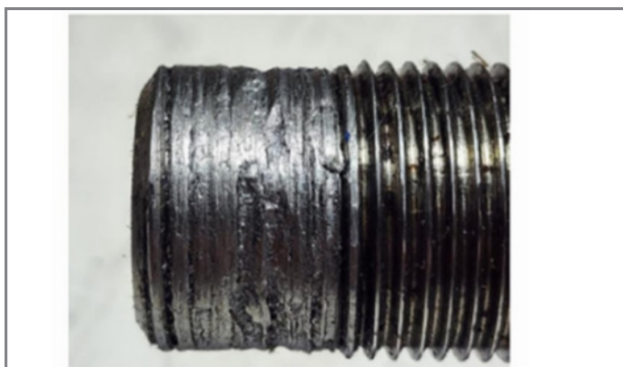
Damage to the wheel drive shaft threads
