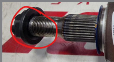
Wheel Drive Shaft Damage
