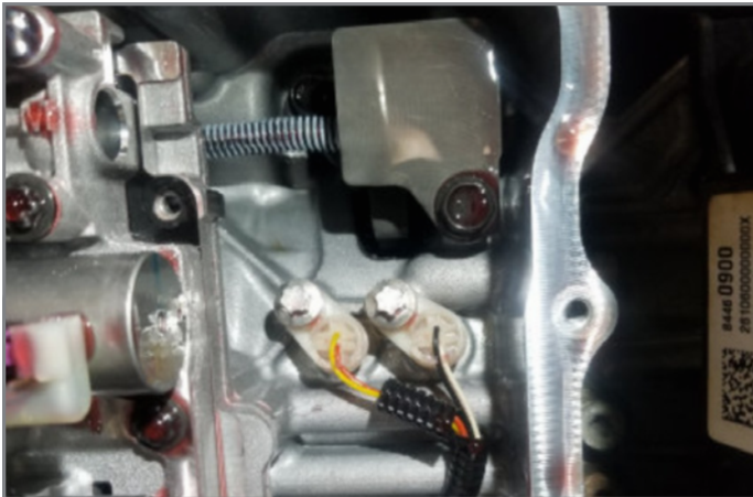
Incorrect speed sensor orientation
