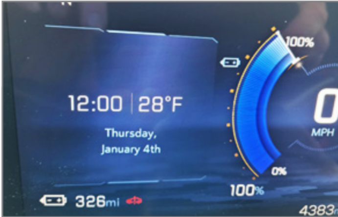
Service Mode is identified by the red icon on the instrument cluster.
