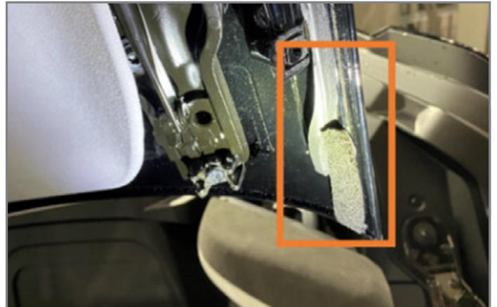
Install a piece of semi-closed EPDM foam.
