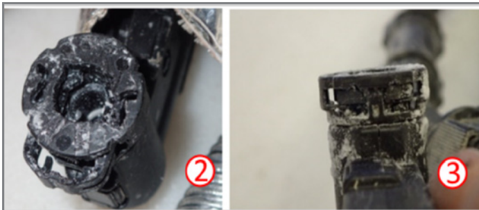
DEF pipe with crystallized DEF.
