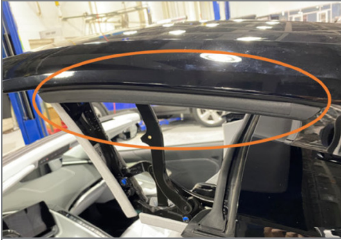
A water leak may be found around the side glass.
