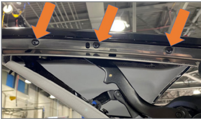
Remove the weatherstrip and weatherstrip retainer
