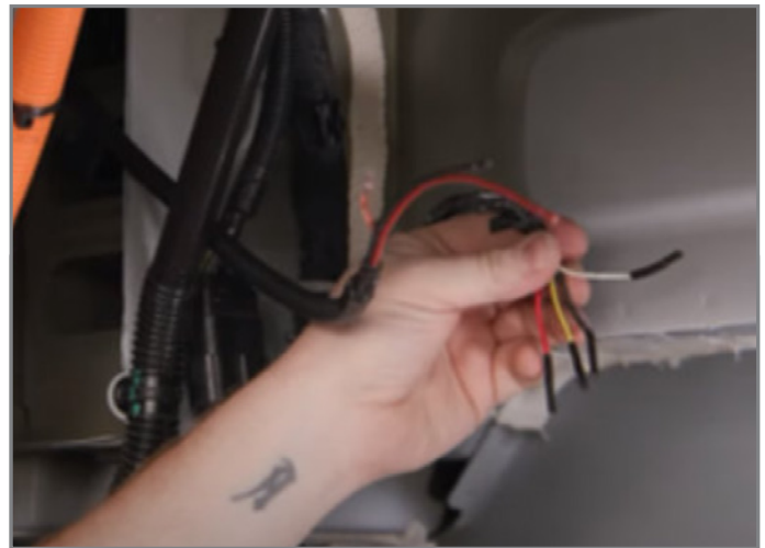
Inspect the 4 wires connected to the main body wire harness.
