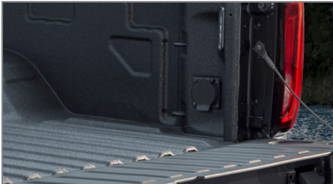
110/120-volt power outlet
