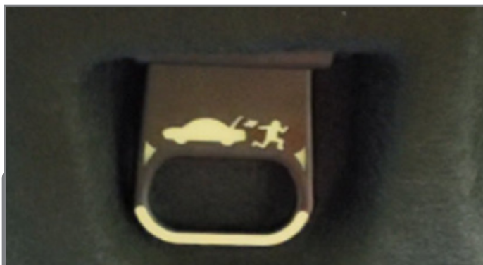
ETR handle not snapped in properly.
