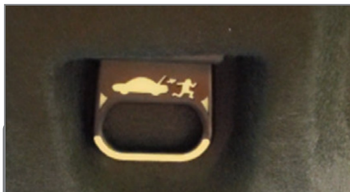
ETR handle snapped in properly.
