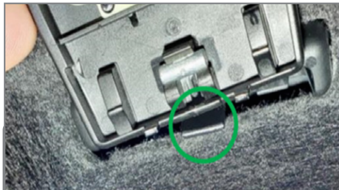
Correct ETR bezel installation with visible bezel tab.
