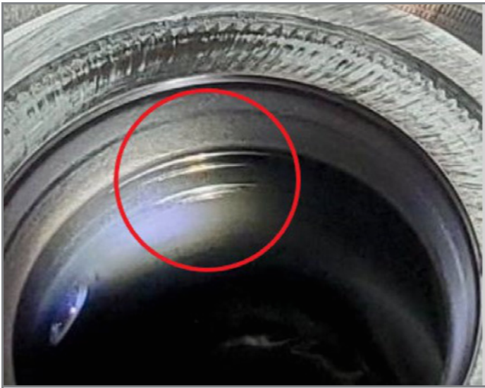
Damage indicates the primary pulley bearing has spun in the bore.
