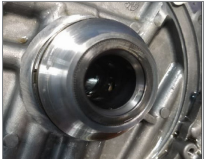
Inspect the pump for signs of wear.
