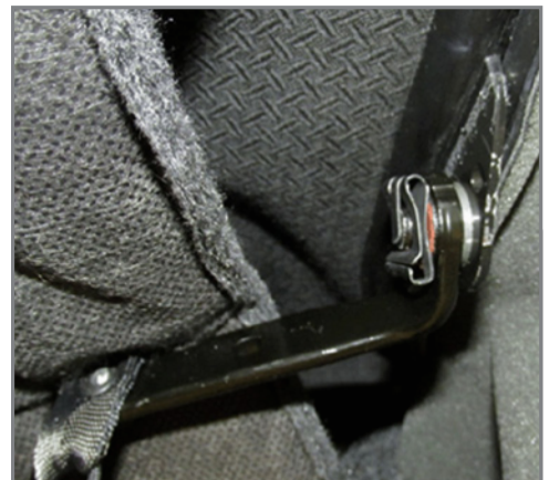
Correctly assembled folding top linkage at the rear glass attachment point
