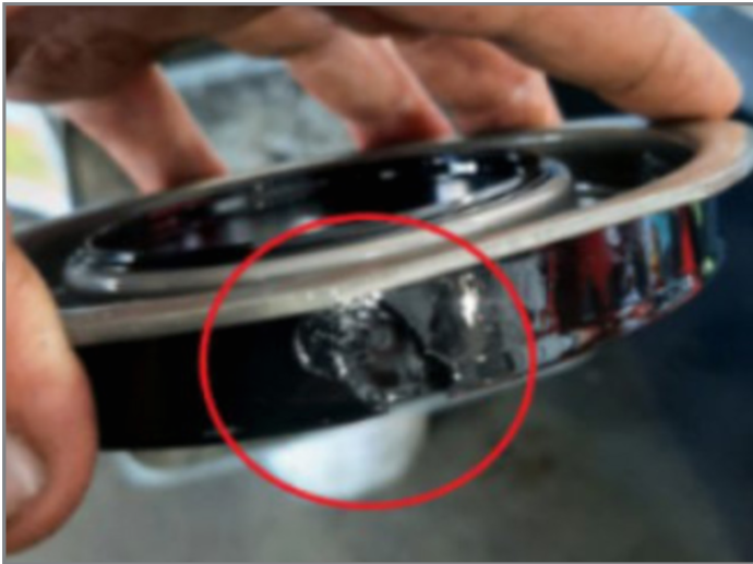
Damage to the forward clutch piston
