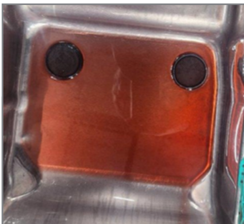
Example that shows good fluid color with no evidence of clutch material.
