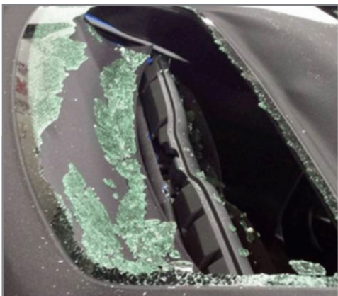
If incorrectly installed, the folding top linkage can create stress on the rear glass.
