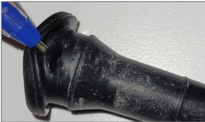
Tire valve stem damage
