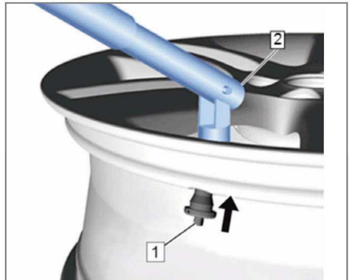
Pull the valve stem (#1) through the valve hole using a tire valve stem installation tool (#2).
