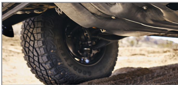
Hydraulic hammer is caused by irregular road surfaces feeding back into the steering gear through the tires and steering linkage.
