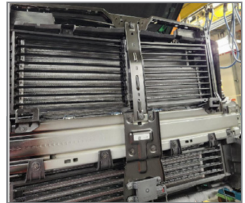
Good front bumper bracket without any damage.
