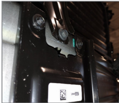
Check for a bend in the lower part of the bracket.
