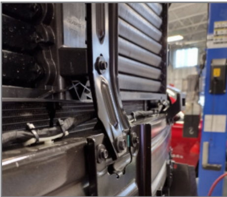
Bent hood-support front bumper bracket
