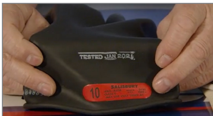
Gloves are stamped with the "tested" date.
