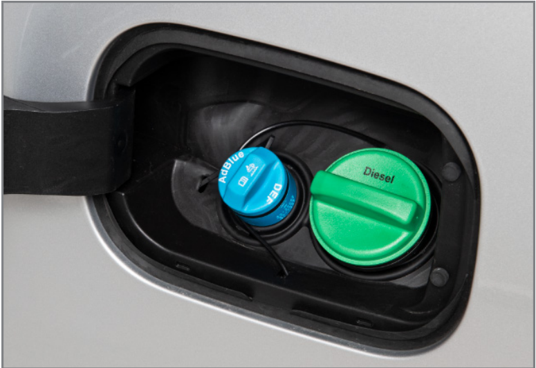
The best time to add DEF to the DEF tank (blue cap) is when a DIC message displays that inducement and speed reduction are imminent.
