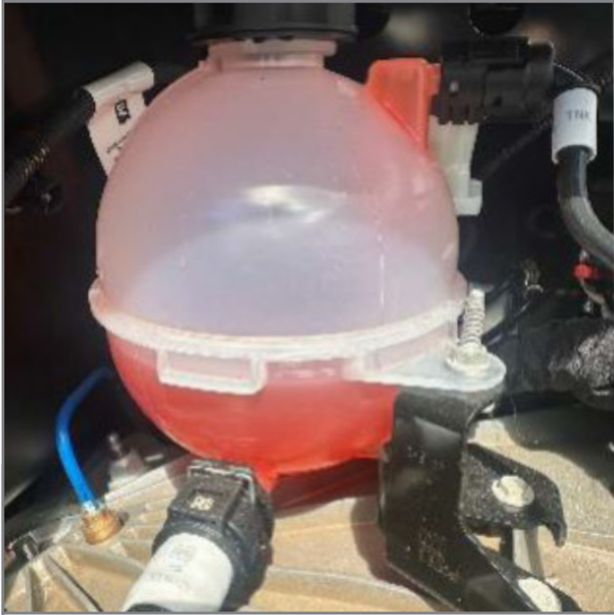
Inspecting the coolant level.
