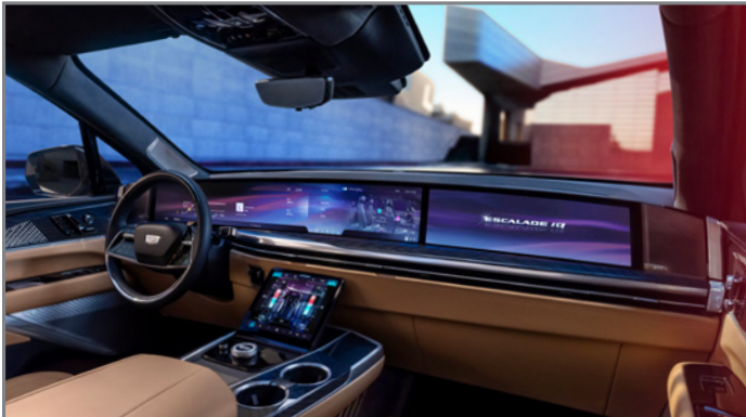
Curved pillar-to-pillar 55-inch-total-diagonal LED display
