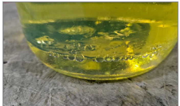
DEF or water in the fuel will sink below the diesel fuel.
