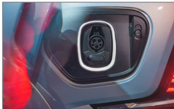
The high-voltage architecture enables 800-volt DC fast charging.
