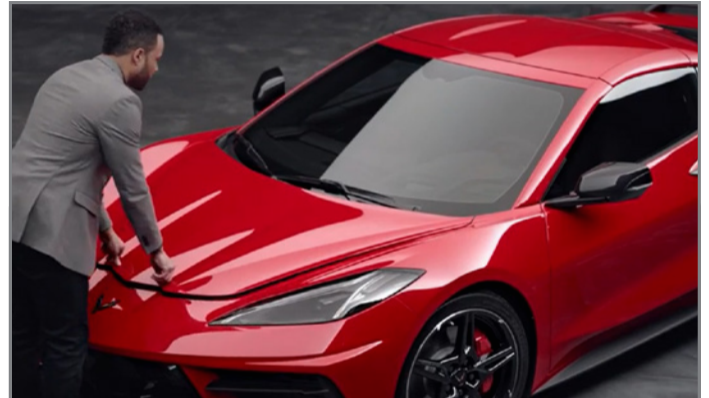
Press down on the hood manually to close it completely before using the manual release cable.
