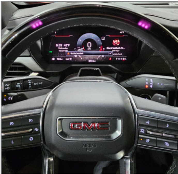
Infrared emitter LEDs on the steering wheel
