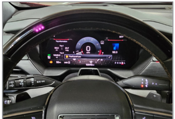
Look for the three illuminated LEDs on each side of the light bar in the steering wheel.
