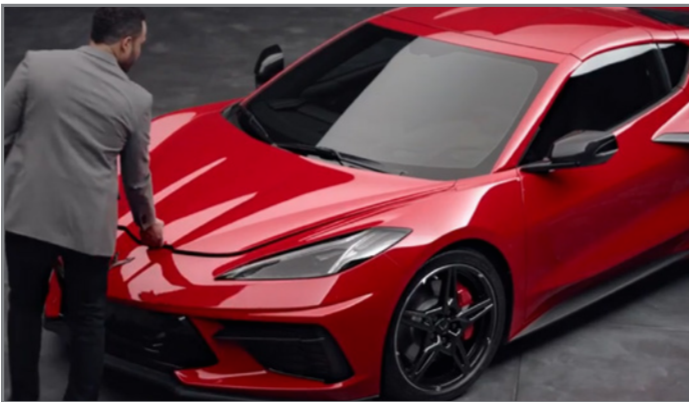
The front compartment hood on may not fully unlatch if the 12V battery is weak.
