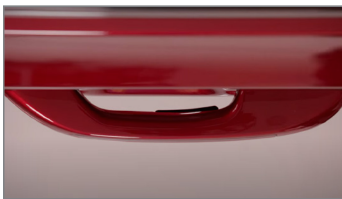
Touchpad on the inside of the exterior door handle
