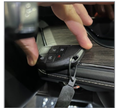
Position the key fob with the buttons facing upward and the base of the fob towards the instrument panel center stack.
