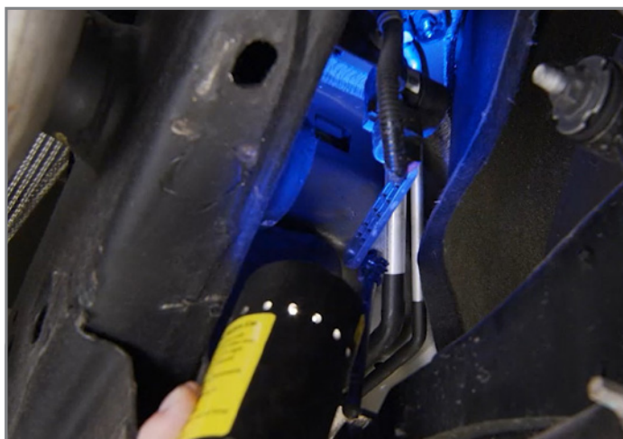
Use the GE-42220 Universal 12V Leak Detection Lamp to help locate leaks in the A/C system.
