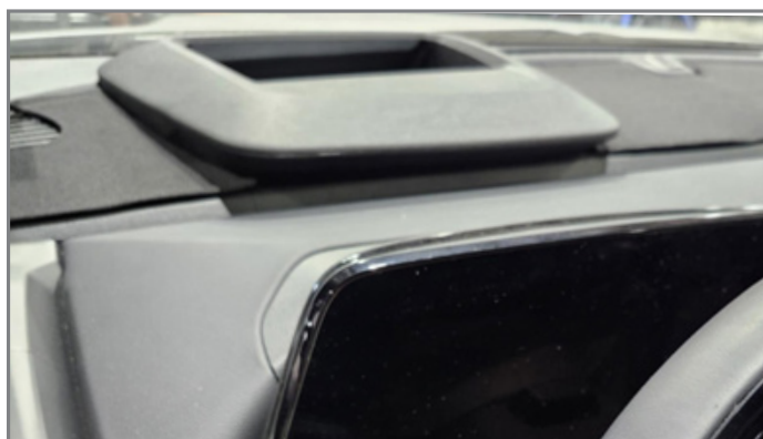
Two-piece dash cover for vehicles equipped with a HUD.
