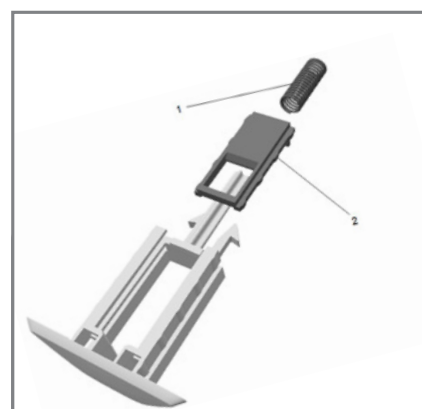
Spring (#1) and latch slider (#2)
