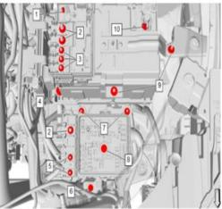
When reinstalling the cables to the fuse, follow the torque specifications listed in SI closely. As you can see in the chart below, they are low in torque.
