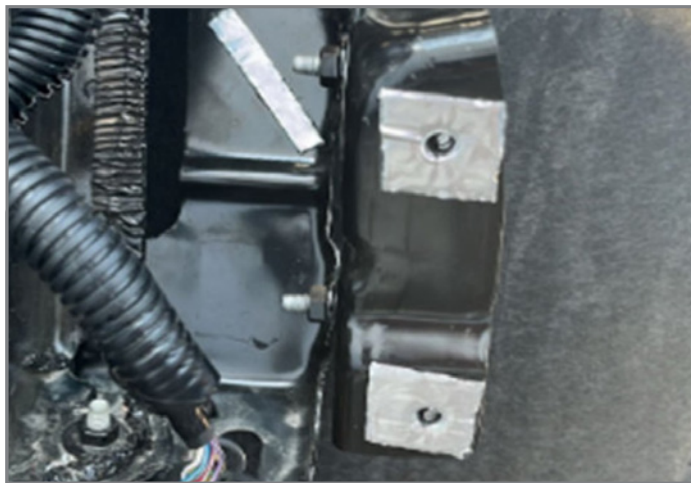
Apply 1-inch squares of foil-backed butyl tape
