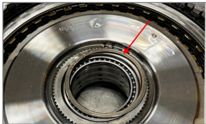
Bulletin #23-NA-197 covers repairs for a dislodged snap ring.
