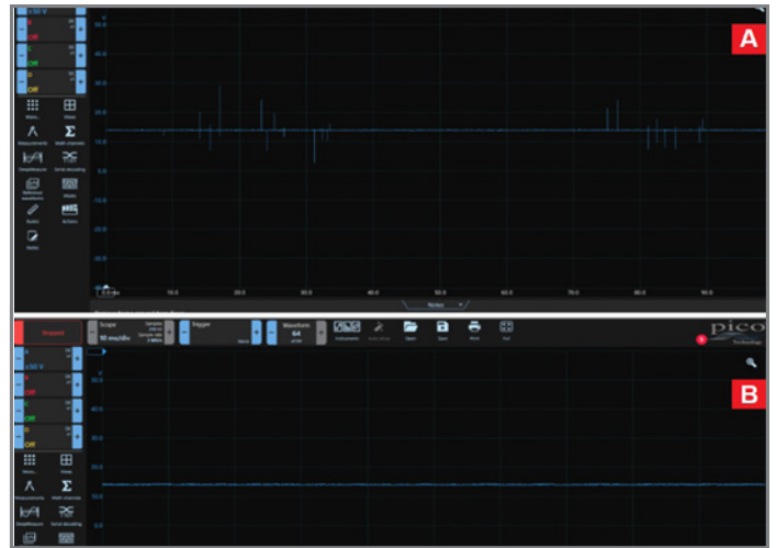
PicoScope reading prior to adding ground cable (A) and after ground cable installation (B).
