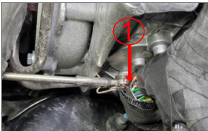
Engine wiring harness chafing at the wastegate linkage.
