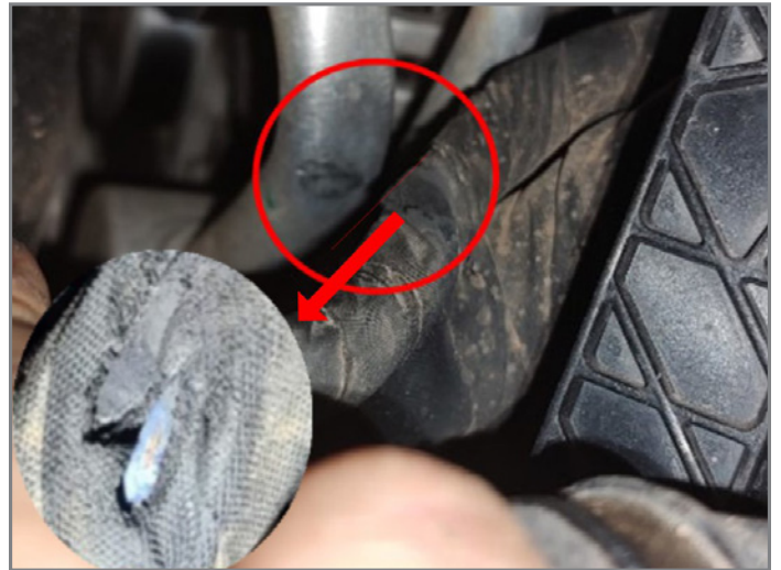
Engine wiring harness contacting the A/C lines.
