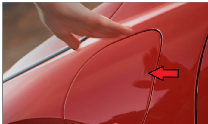
Small oval-shaped protrusion indicates where to press to open or close the charge door.
