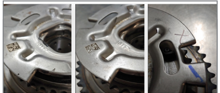
Check for excessive clearance of the actuator ring.
