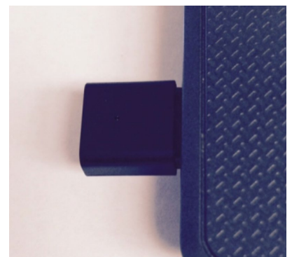
Wireless 802.11 dongle plugged into the PC.
