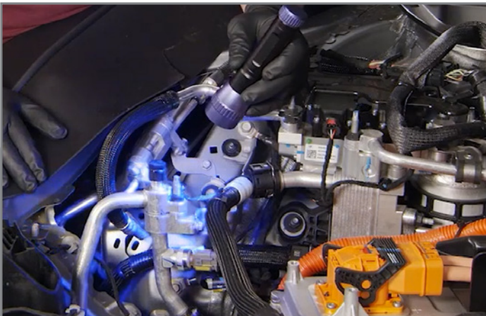
Updated A/C leak diagnosis requires a different fluorescent dye process than used on earlier systems.
