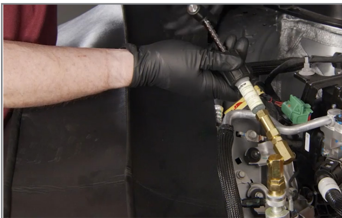
Injecting dye into the A/C system.
