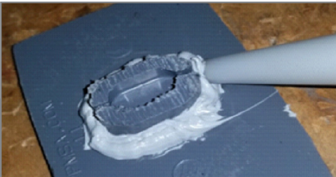
Cut down the stem and apply a small amount of RTV sealer.
