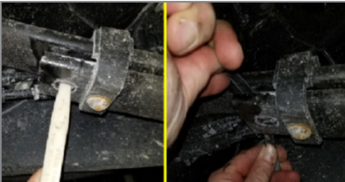
Push up on the insert and cut off the stem.
