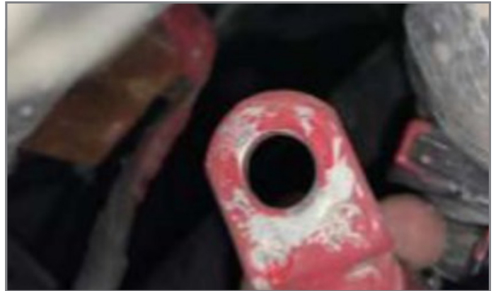
Inspect red anti-corrosion paint between the eyelet and engine block.
