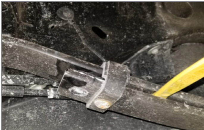
The left rear leaf spring insert may have been contaminated during refueling.
