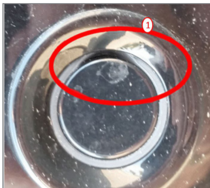
Silicone ring not properly installed.
