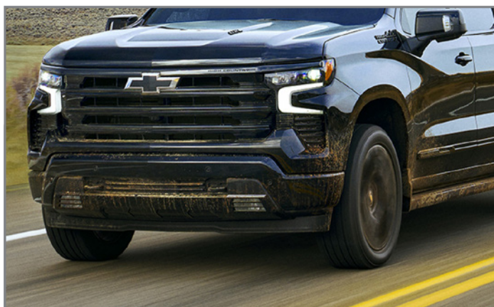
A sensor obstructed by mud on the bumper may cause a false alert.
