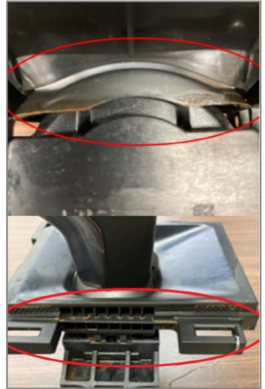
Evidence of liquid contamination
