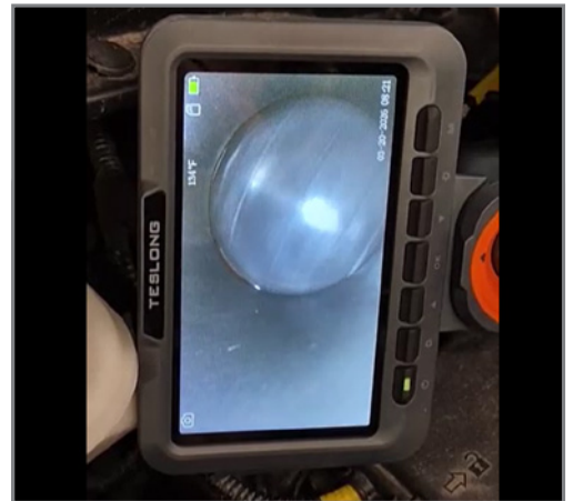
The CCV ball valve should cycle smoothly.
