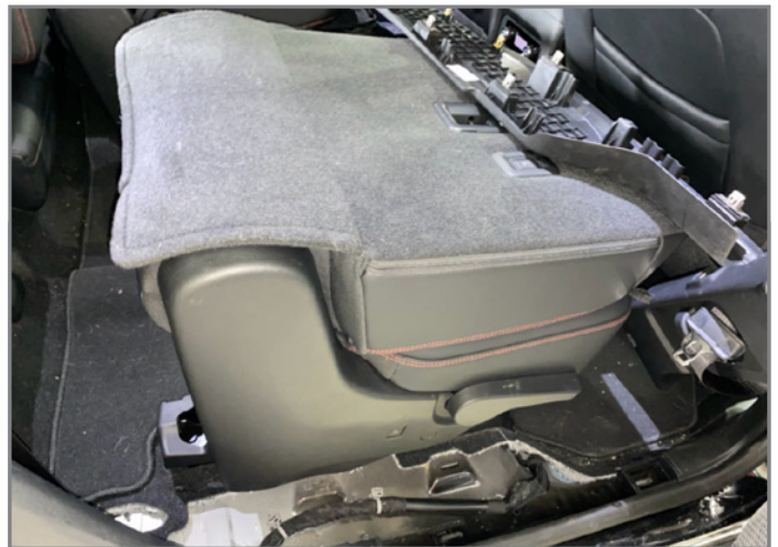
Remove the necessary interior trim pieces to access the Ethernet cable.
